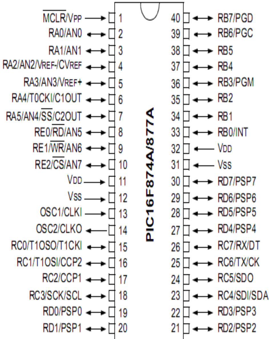
Figure 1.2: Pin configuration of PIC 16F877A (Micro-Controller)
