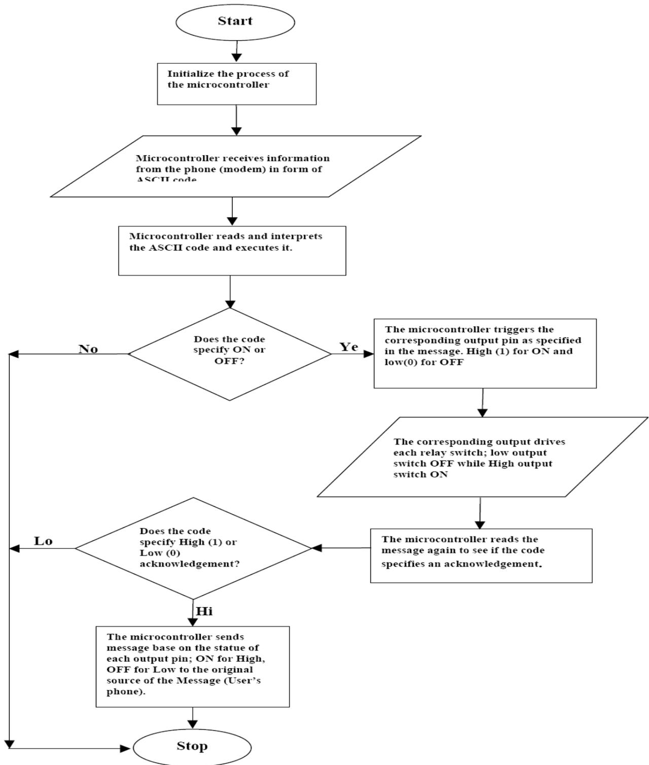
Figure 1.5: Flow diagram of the program activities of the microcontroller
