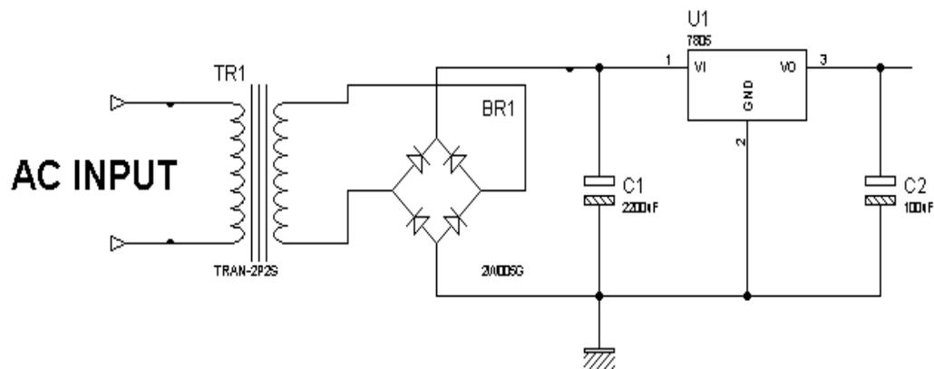
Figure 1.1: Rectifier Circuit
