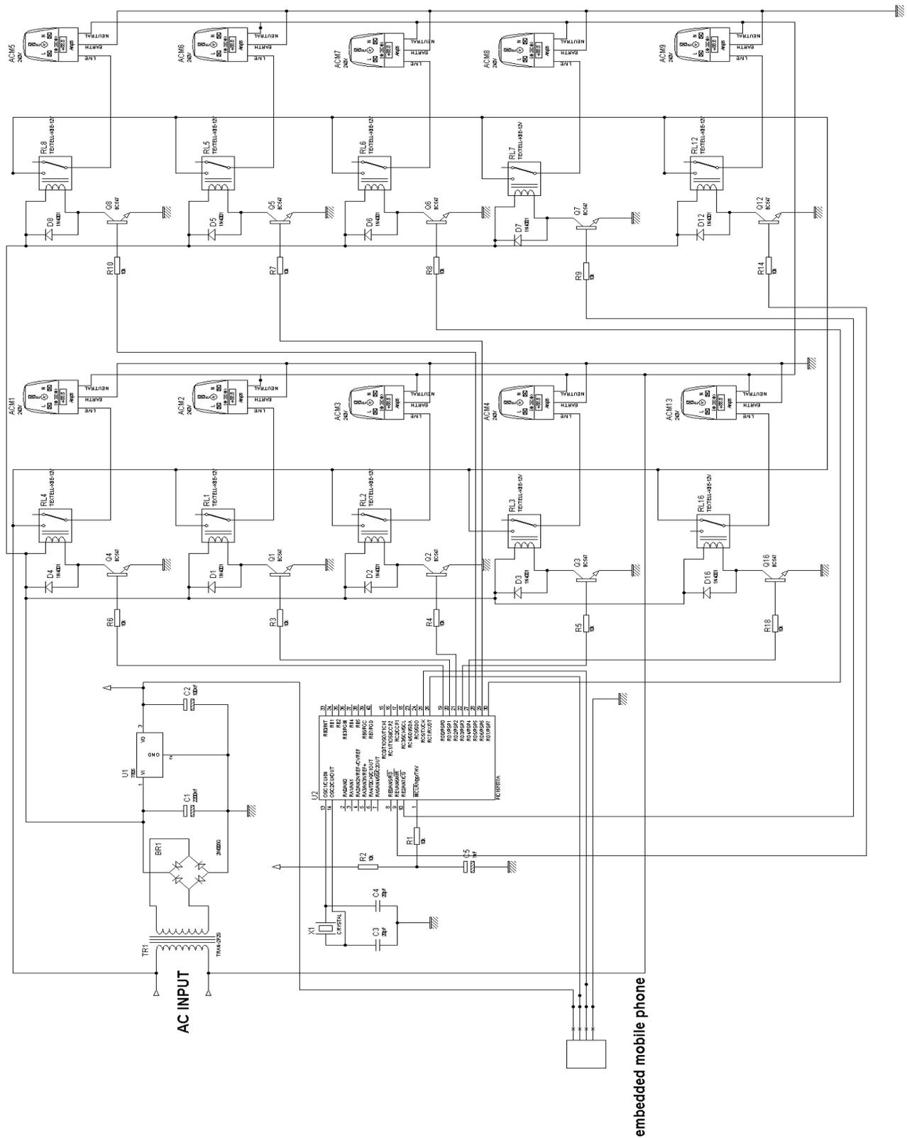
Figure 1.6: Circuit diagram of the GSM based household power management system
