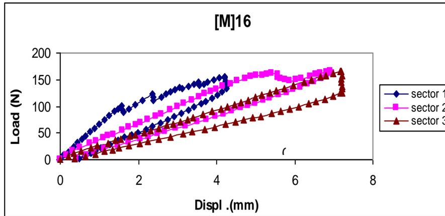
Figure (2) Load – Displacement curve in woven roving glass fiber /Epoxy composites
