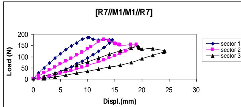
Figure (8) Load –Displacement Curve for [R7//M1/M1//R7]
