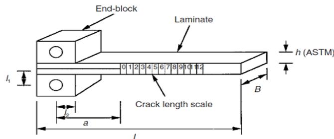
**Figure (1) Specification of unloaded DCB specimen**
