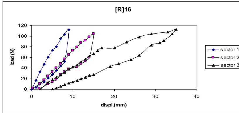
Figure (4) Load – Displacement curve in random glass fiber /Epoxy composites
