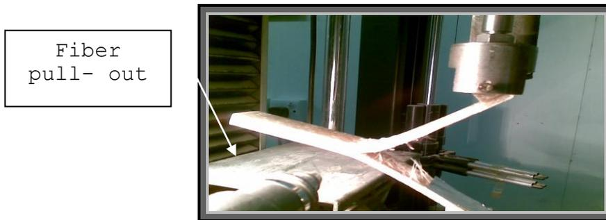
Figure (6) broken fibers pulled out from the resin as an evidence of fiber bridging.
