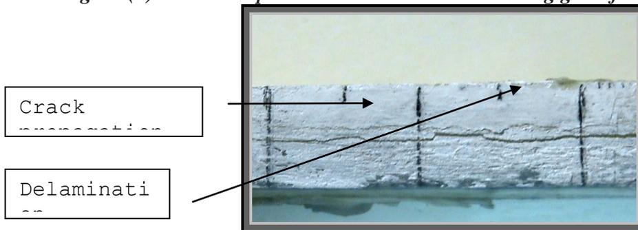
Figure (3 ) DCB test for woven roving glass fiber /Epoxy composites
