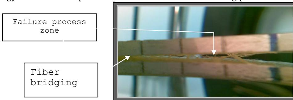
Figure (5) fiber bridging for random glass fiber /epoxy composites.
