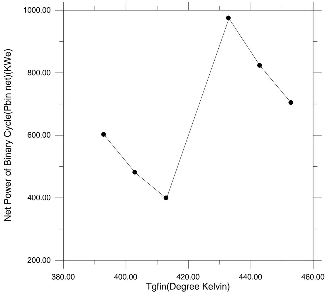
Fig.(3) Variation of Temperature of Geothermal Fluid at the Entrance with Net Power of Binary Cycle.
