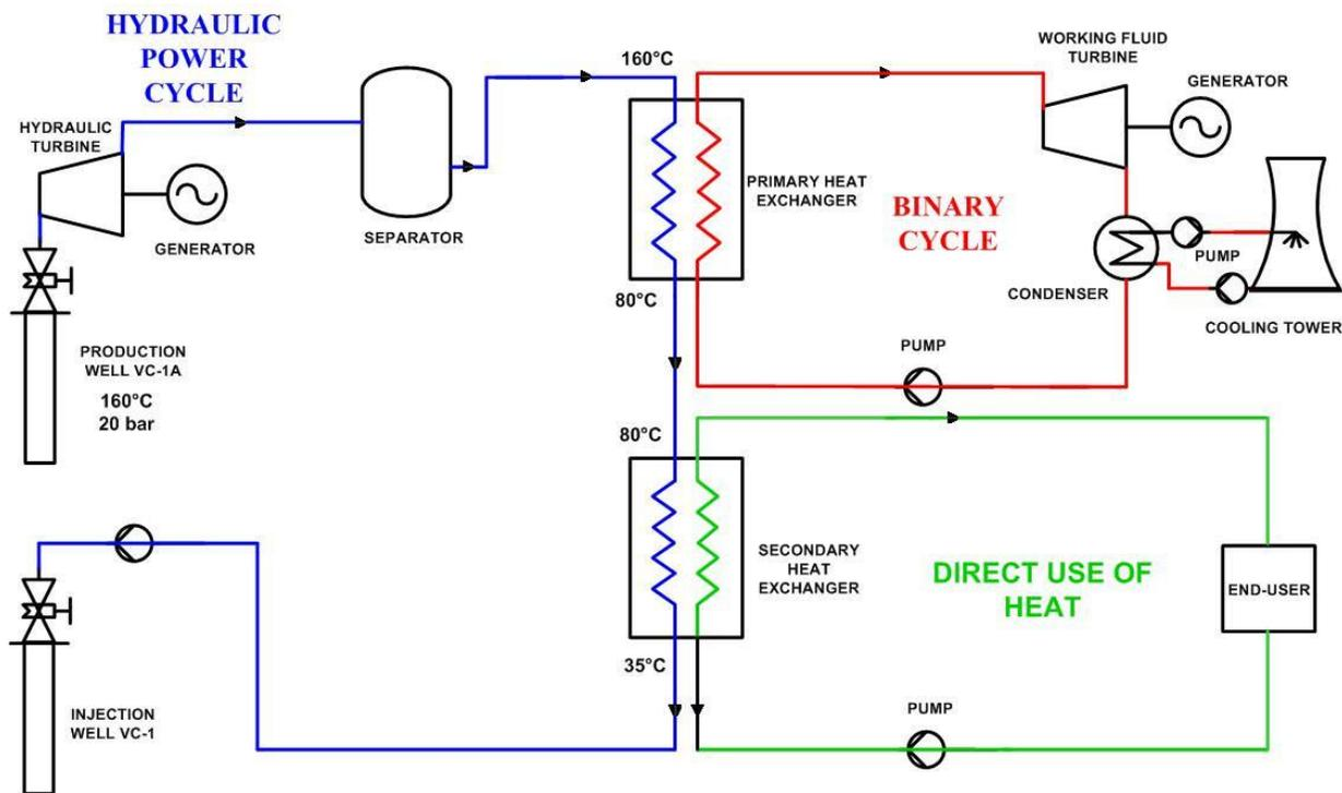
Fig. (1) Scheme of Geothermal Power Production [Olurvody,1984]
