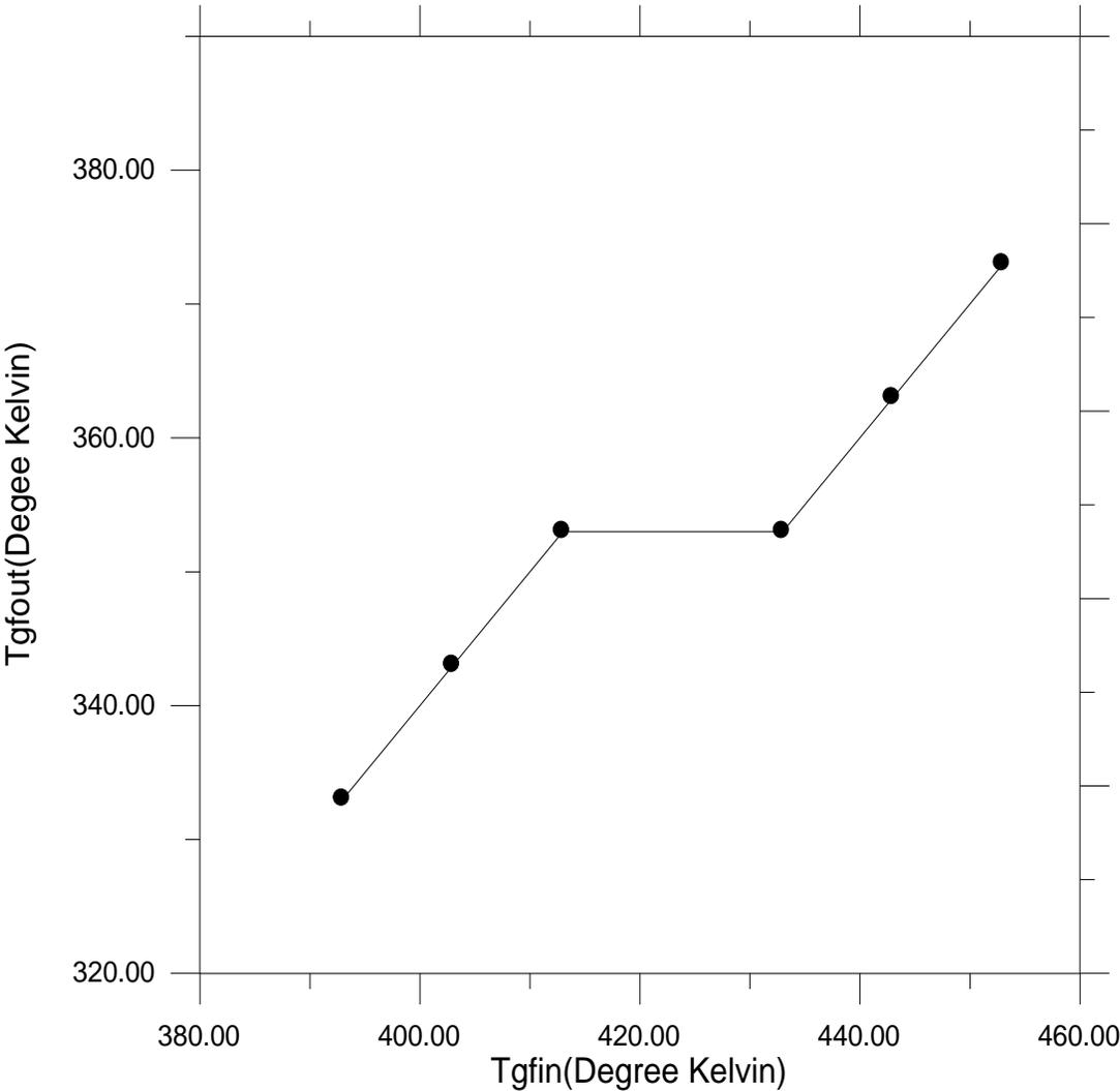
Fig.(2) Variation of Temperature of Geothermal Fluid at the Entrance(Tgfin) with Temperature of Geothermal Fluid at Exit(Tgfout).
