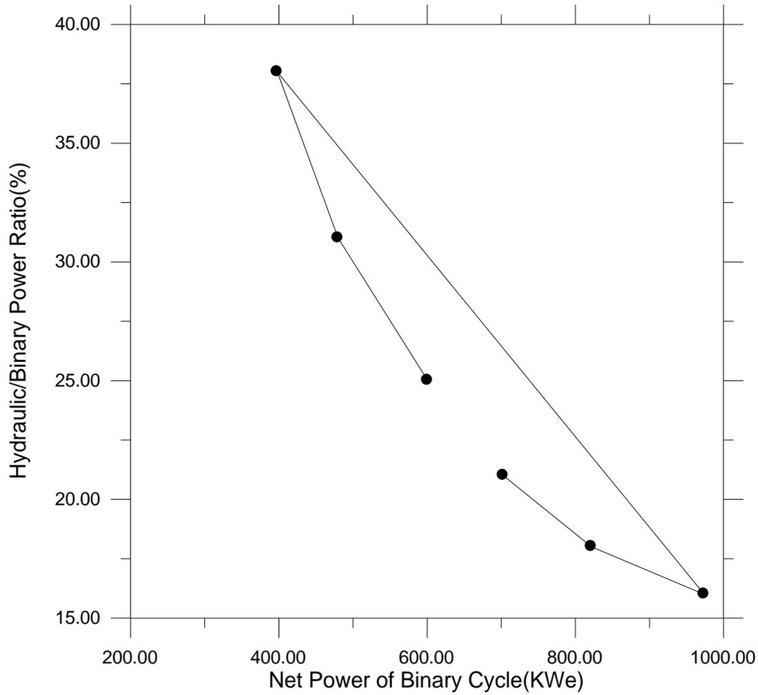
Fig.(5) Variation of Hydraulic/Binary Power Ratio with Net Power of Binary Cycle.
