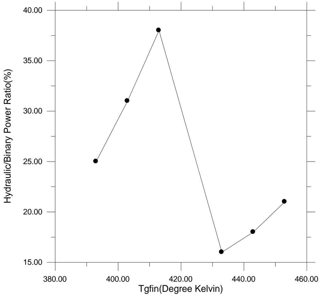
Fig.(4) Variation of Hydraulic/Binary Power Ratio with Temperature of Geothermal Fluid at the Entrance.
