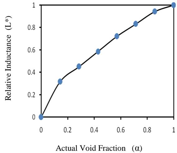
**Figure(3): Calibration curve for void fraction using air and water**
