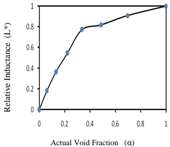
**Figure(4): Calibration curve for void fraction using wood and water**
