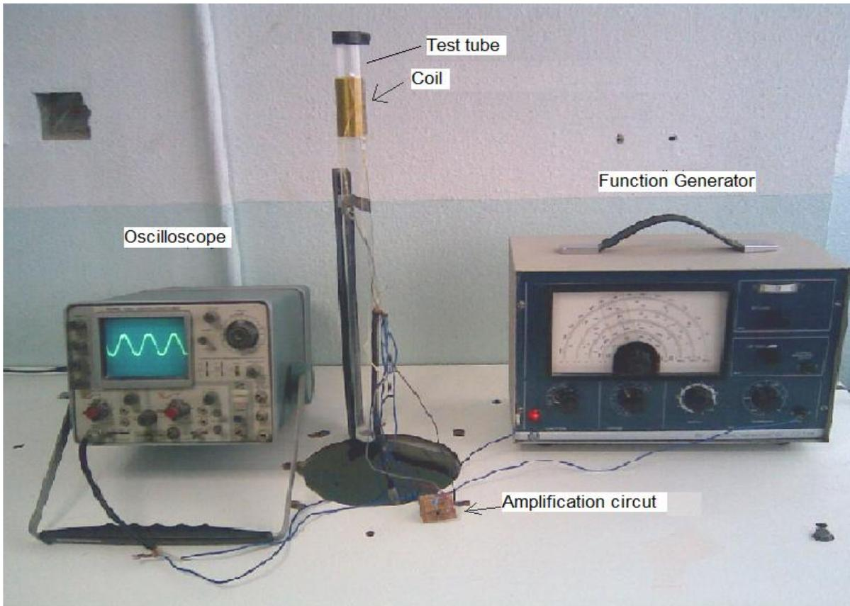
Figure (1): The experimental arrangement of the auto-transformer used for void fraction
