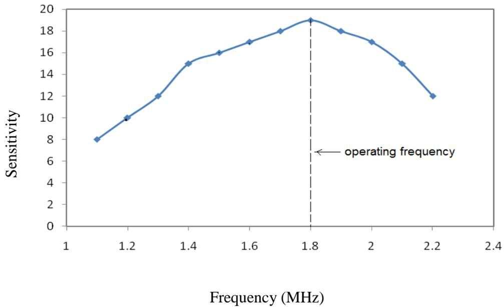
Figure(2): Experimental determination of maximum sensitivity of the auto-transformer
